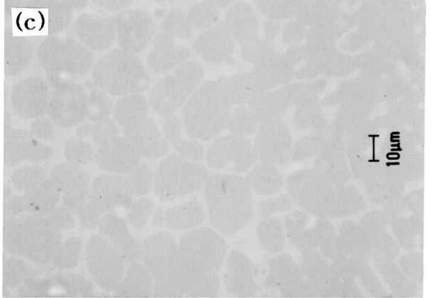
Figure 7 Optical micrographs show the as-cast microstructure of Pd-In system alloy (before the tarnish test) (a) 40Pd-29In-26Ag-2Zn-Au-2Cu (wt.%) (b) 40Pd-29In-25Ag-2Zn-2Au-2Cu (wt.%) (c) 40Pd-29In-23Ag-3Zn-3Au-3Cu (wt.%).
